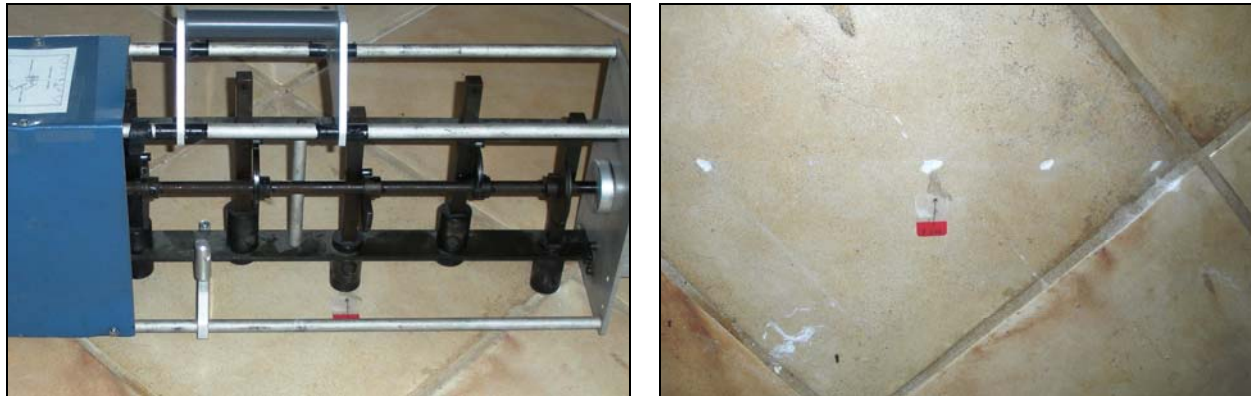
Fig 3 - Field Impact Insulation Test (FIIC) photographs: before (l), after (R).
