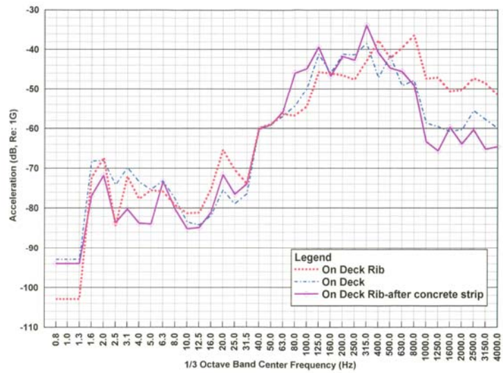
Fig. 12 - Vibration measurements after concrete strip installed.
